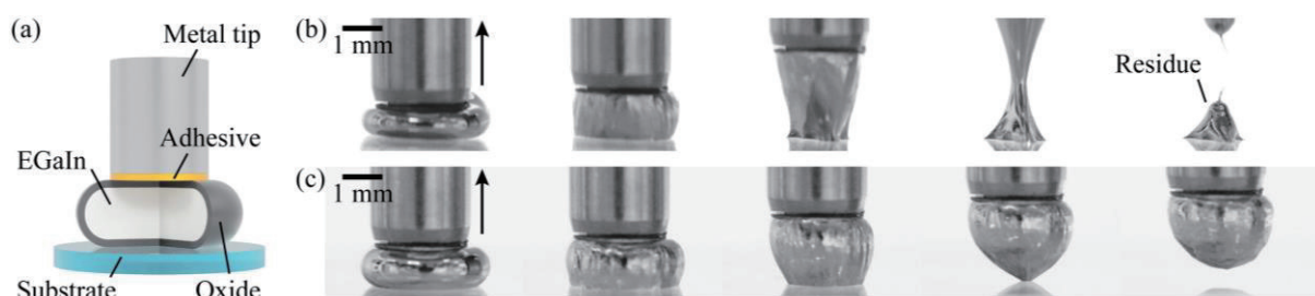
Figure 1. Investigation of contact line motions of oxide-coated EGaIn droplet. (a) Schematics of an experimental setup. (b) Typical contact line motion with metallic residue. (c) Instance of contact line motion without residue.
